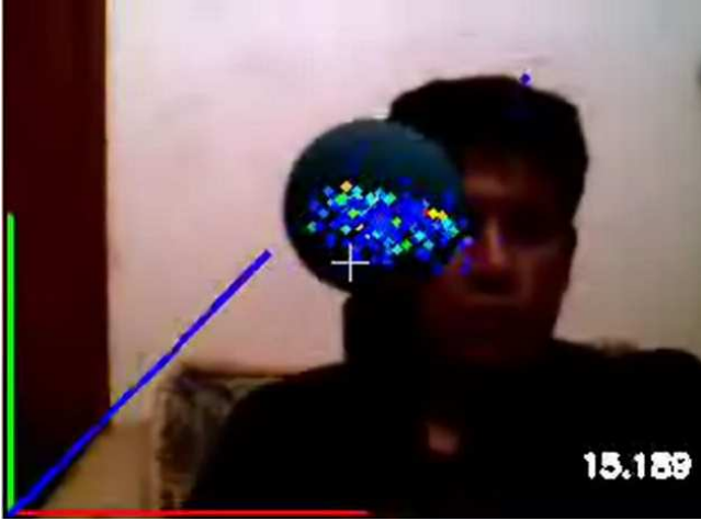
Fig. 3. An example of visual tracking of a blue ball. The dots over the ball represent the different estimates of the ball position (x, y) given by the particle filter. The axis represent the ball position in 3-D; the horizontal axis is the x coordinate, the vertical is y , and the third one at approx. 45 degrees represents the depth or z .
